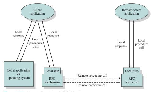
Figure 16.14 Remote Procedure Call Mechanism
