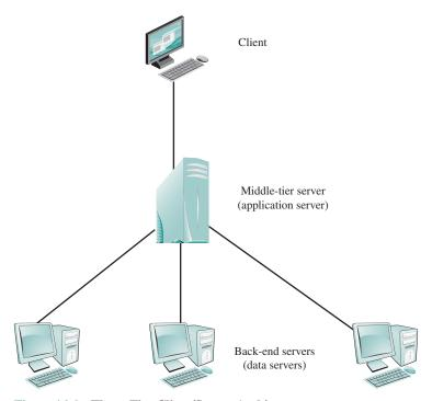
Figure 16.6 Three-Tier Client/Server Architecture
