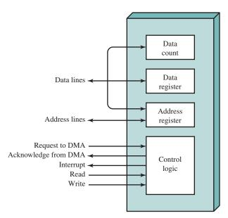
Figure 11.2 Typical DMA Block Diagram
