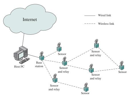
Figure 13.10 Typical Wireless Sensor Network Topology
