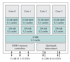
Figure 1.20 Intel Core i7 Block Diagram
