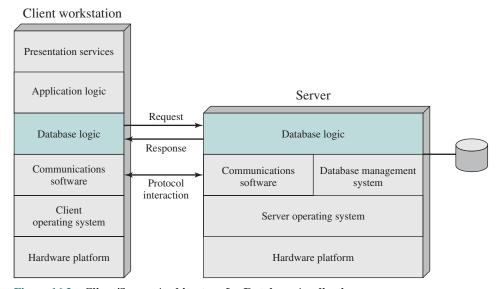
Figure 16.3 Client/Server Architecture for Database Applications
