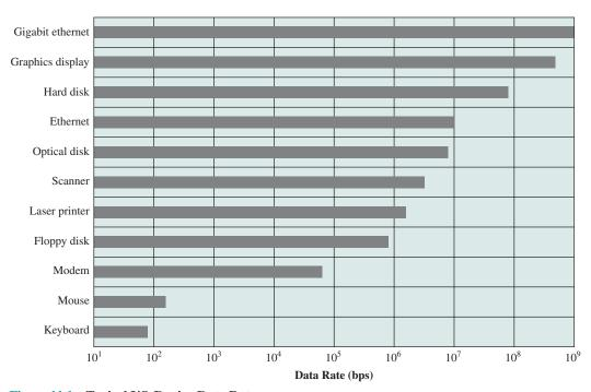
Figure 11.1 Typical I/O Device Data Rates
