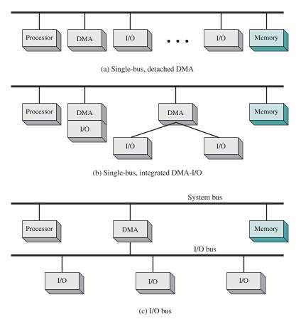
Figure 11.3 Alternative DMA Configurations
