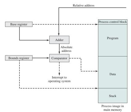
Figure 7.8 Hardware Support for Relocation
