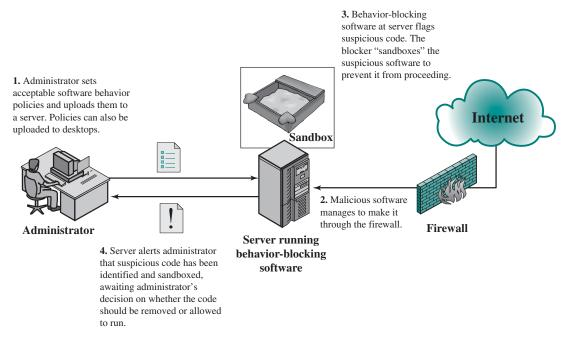
Figure 15.10 Behavior-Blocking Software Operation
